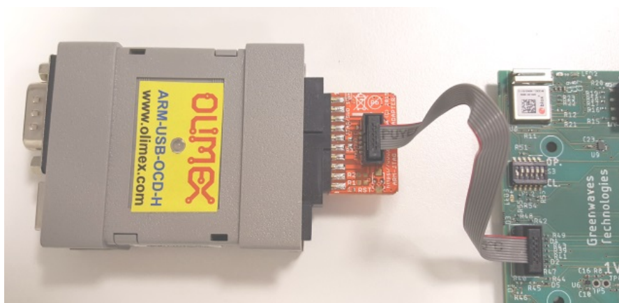
Fig. 3 – OLIMEX probe with JTAG-20-10 adapter
