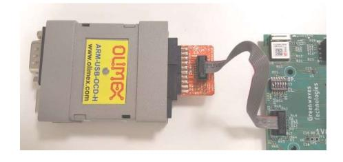
Fig. 2 – OLIMEX probe with JTAG-20-10 adapter
