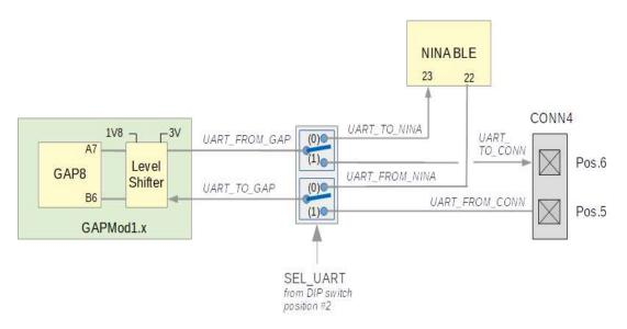
Fig. 4.a – UART Sharing scheme on GAPPoc A V0.1
