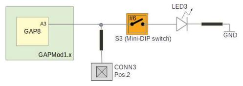
Fig.6 – Sharing of GAP8 pin A3: external connector vs. on-board green LED
