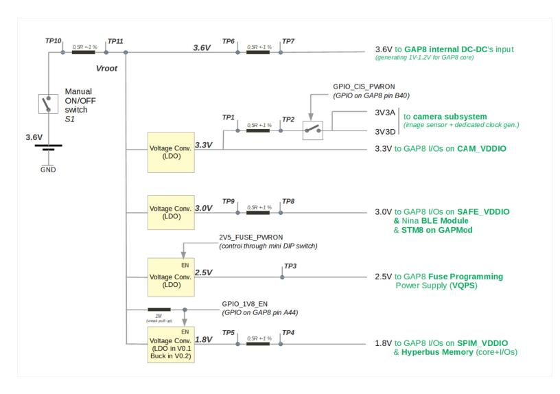
Fig. 3 – On-board power supply generation and control (notional)
