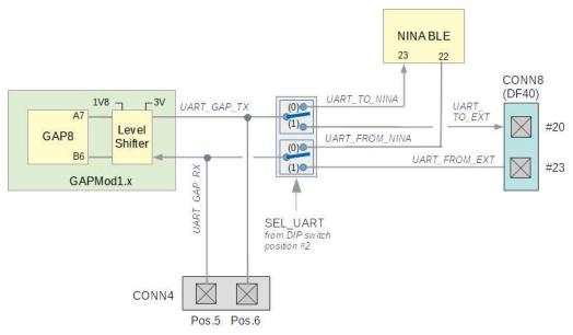
Fig. 4.b – UART Sharing scheme on GAPPoc A V0.2
