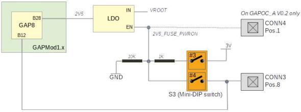
Fig. 5 – Control scheme for 2.5V power supply
